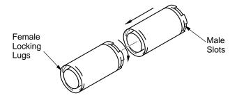
Figure 8 - Vent Pipe Connections
